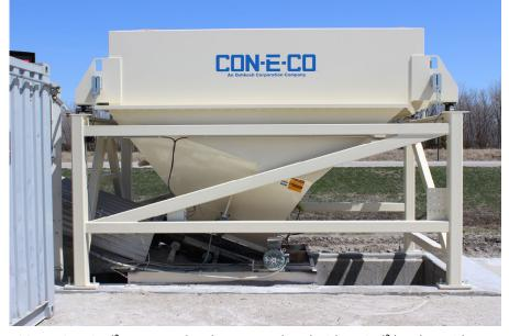
**SOLUTION:** 8 yd<sup>3</sup> aggregate batcher was replaced with a 12yd<sup>3</sup> batcher with the ability to add a 100yd<sup>3</sup> aggregate storage bin with 3 compartments.
